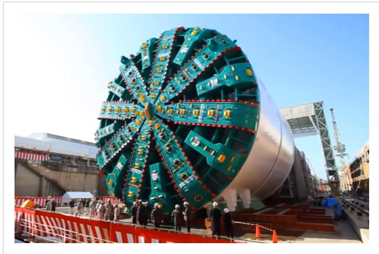
**Design-build with early contractor engagement applied to the Seattle SR99 Alaskan Way highway project and its 17.5m diameter EPBM excavation system**
